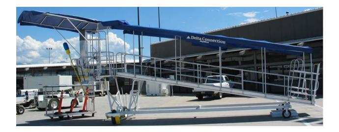
The Swinging Gate Ramp (SGR) is designed to allow passengers to board and deplane without traversing aircraft steps.
